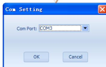
The port indicator at the bottom of the config software will turn green when the Com port is correctly set.
