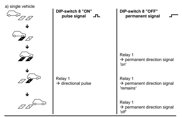
Evaluation of the direction signal in the opposite direction is done in the same way. In case of a loop break resp. –closing, the system switches to the presence detection mode for the time of the failure. A soon as the loop is occupied, a permanent signal will be emitted by the relay of the intact loop channel.
