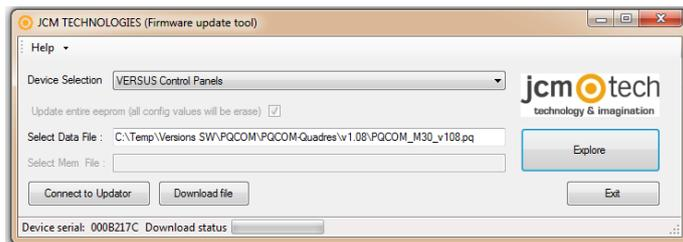
5 - Press the button "Download file" to download the chosen file to the device Updator. Wait until you finish the download process (the state is indicated by the bar "Download Status"). Once the process is finished, it is indicated in the bottom of the window by "Download OK".
