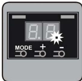
It is only available to enter standby mode if the door is not in movement and if there is no error activated.
