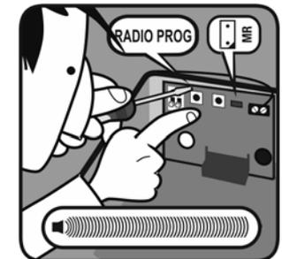
PRESS RPROG PUSHBUTTON LED TURNS OFF & END PROG
