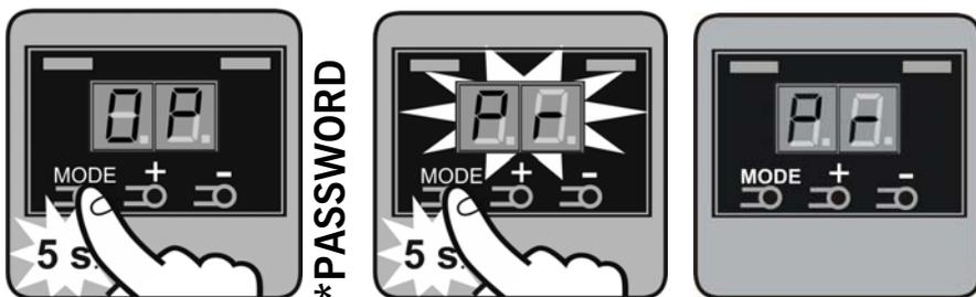
Being in “Door state indication” mode, press the MODE button during 5 seconds. PA will appear on the display indicating that the control panel has entered programming mode. Once finished the programming of the maneuver, the control panel will exit this mode automatically after 30 seconds.
