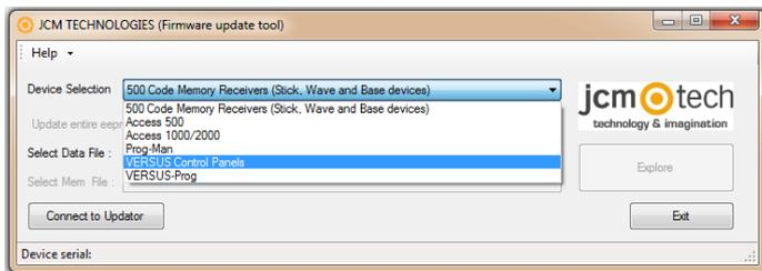
3 - Press the "Connect to Updator" and if the connection is correct, at the bottom of the window you will see the serial number of the Updator (Device serial).
