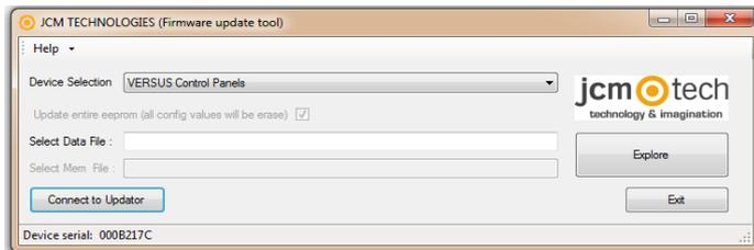
4 - Using the "Explore" to choose the firmware file corresponding (with extension \*.pq).
