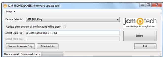
5 - Press the button "Download file" to download the chosen file to the device Updator. Wait until you finish the download process (the state is indicated by the bar "Download Status"). After the process, in the bottom of the window "Download OK" is indicated.
